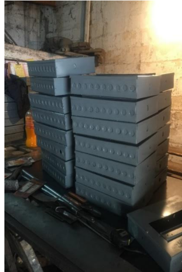
Fig. 5(b): Completed electrical distribution boxes
