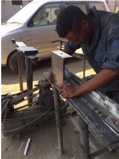
Fig. 5(a): Tin smith folding parts of an electrical distribution box.
